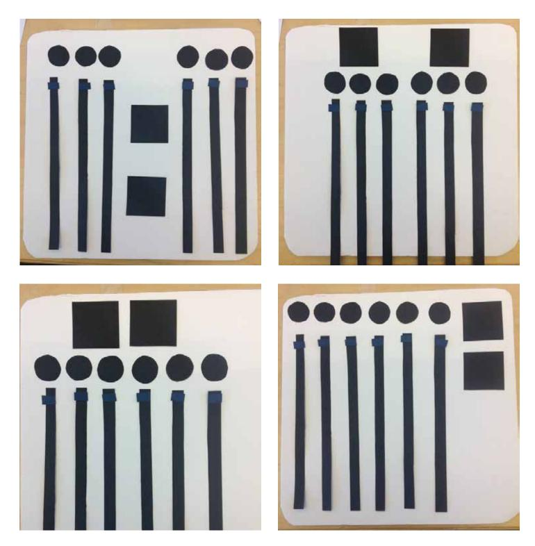
This visualization exercise examines a variety of control and track configurations for the device. Included are a switch for each track (circle), temperature control and vac gauge (squares), and sliders (in blue).
